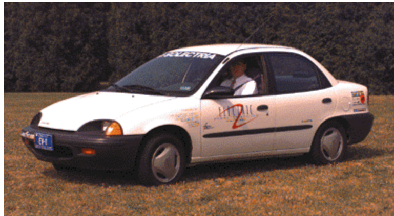
PHOTO 1 1995 Subcompact Electric Vehicle is retrofitted General Motors Geo Metro 4-door sedan
